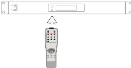
**Distance:** within 7m from the front of the remote control sensor.
